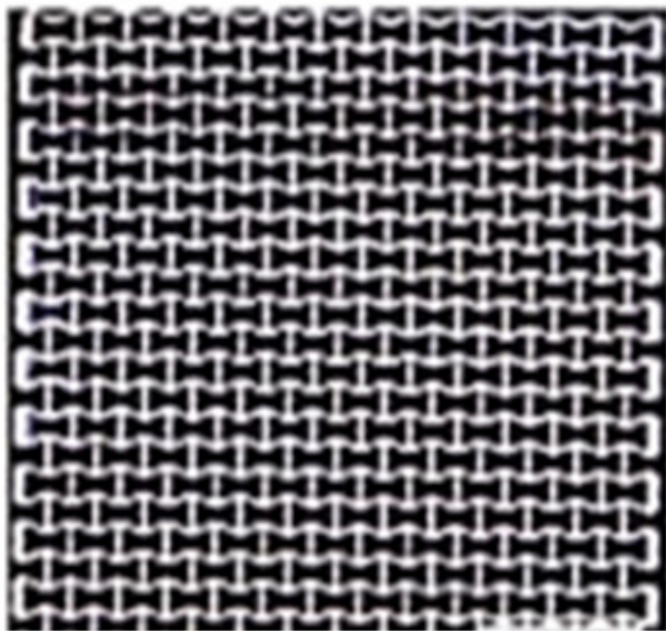
Micromachined re-entrant pattern on metal sheet
